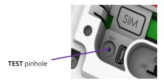
The CP LEDs flash and the CP beeps three times. The CP is restored to factory settings.
