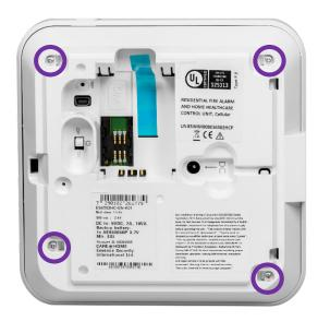
6. Use a flat screwdriver to press apart all the latch tabs, and remove the bottom of the CP from the front. The latch tabs are beside the screw holes.
