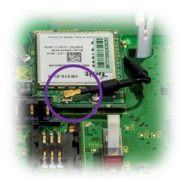
8. Carefully connect the external antenna adapter to the circuit board, to where the internal antenna was connected, as shown in the following image.
