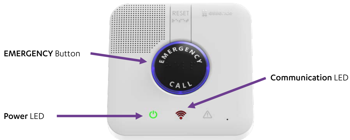
Figure 7: Powering Up the Control Panel
