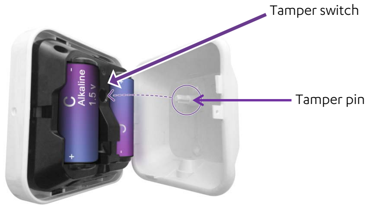
Figure 27: Aligning the Tamper Pin and Switch to Close the VPD
