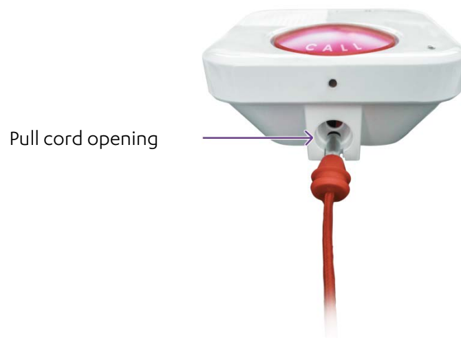
Figure 30: Inserting the Pull Cord
